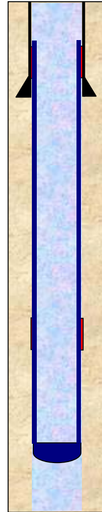
Pop-Out Leaving Open Hole Liner
